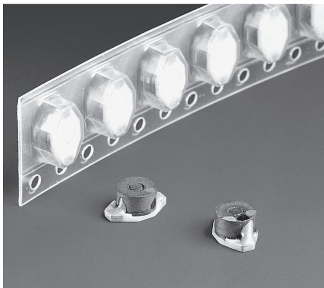
The Coilcraft DT1608 Series represents the ultimate in cost-effective, miniature power inductors. The DT Series is magnetically shielded and the materials used provide natural heat sinking. This allows these parts to be used at relatively high currents. Even at 150% of rated current, the temperature rise is less than 15°C.
